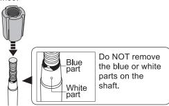
finsert the lower shafts into the grip and turn clockwise to lock in place.
