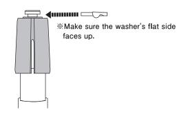
Place your weight on the pole to see that the stopper is performing as intended and have securely locked the shafts in place.
