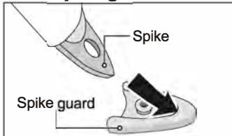
First, insert spike tip into the cover, then secure the whole spike.
