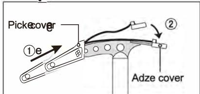
Slide on the pick cover first, then attach the adze cover.
