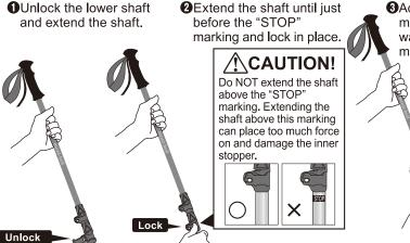
Adjust the length of the middle shaft in the same way. Use the scale on the middle shaft as a reference.
