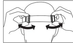
Slide the adjuster parts on the headband to the left or the right to adjust the fit. Sliding the adjuster parts outwards will tighten the fit, while sliding them towards the center will loosen the fit.
