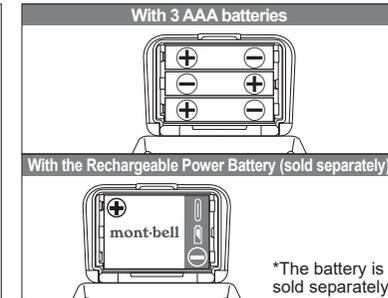
② Insert either three AAA batteries or the Rechargeable Power Battery (sold separately) into the slot, ensuring the + and - orientations are correct.
