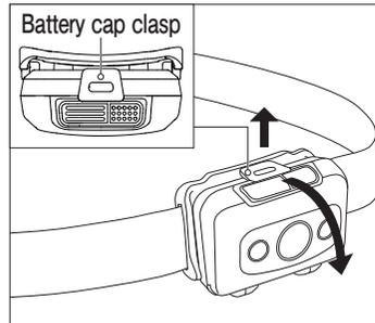
① Lift the battery cap clasp and open the headlamp.
