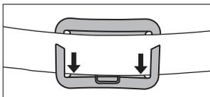
① Insert the lower end of the headlamp into the headband holder.
