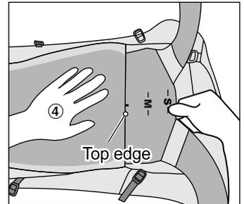
① Measure your torso length based on the figure above. The shoulder harness of this product is adjustable to accommodate the following torso lengths.
