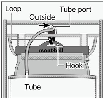
Attach the hook on the slide lock bar of the Trail Water Pack to the loop located at the top inside the main compartment. Pass the tube through the port to the outside of the pack.
