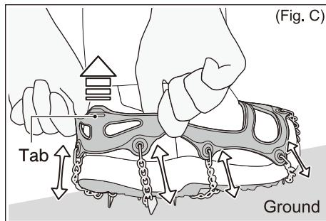
**CAUTION** Make sure to install and use this product correctly when wearing. If the spikes are facing towards the soles of the shoes (product is mounted upside down) or if the chain is loose, the product will not exert its full traction, which is dangerous.
