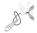
(11) Pull the end of the wire lace tightly to for a knot.
