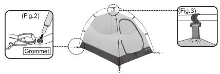
3 Insert the ends of the pole to the grommets (Fig. 2).
