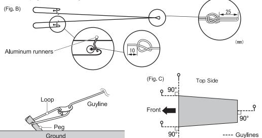
**6** If using the Zelt Pole Set, fit the anchor ring over the end of the pole and then place the guyline loop on top. Then stand the pole up straight. If using trekking poles, use the anchor loop instead.
