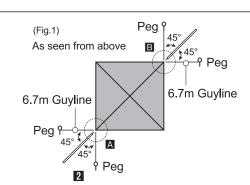
2Stake pegs on two opposite corners (see Fig. 1). Loop guylines around pegs.
