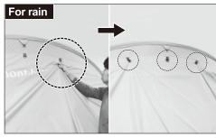
During rain, connect the 3 toggles on the middle of the side panel to the rings on the top of the Astro Dome. This will angle the side panel and prevent water from pooling.
