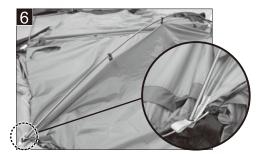
Attach the pole hooks on the ceiling to the short pole.
