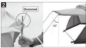
Seat the grommet on the end of the side panel on top of the pole. Loop the guyline around the top of the pole and pull it down at a 45° angle and stake it with a peg.
