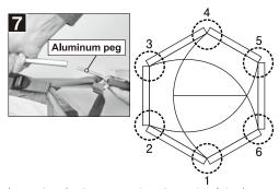
Insert the aluminum pegs into the ends of the long poles (6 places).
