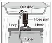
Hang the hook connected to the Trail Water Pack from the loop on the inner hook as shown in the figure.
