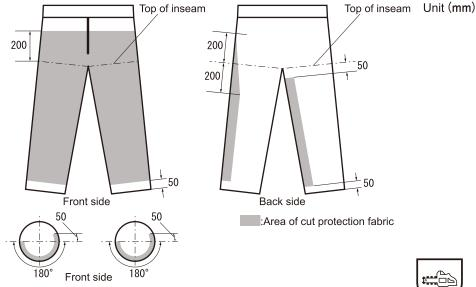
The pictogram according to ISO 7000 indicates that this product provides cut protection against chainsaws. Class 1: chain speed of 20m/s, equivalent to the speed of a 50cc chainsaw operating at full speed when cutting wood.
