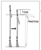
●Adjust the length of the leash to match the length of the ice axe as shown. When doing so, make sure the head loop is at least 11cm in length.
