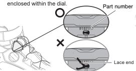
(§) Push the dial into the bayonet until it clicks into place. Check that it's working correctly by following the instructions on page 6.
